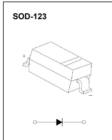
**Maximum Ratings and Electrical Characteristics, Single Diode @Ta=25°C**
